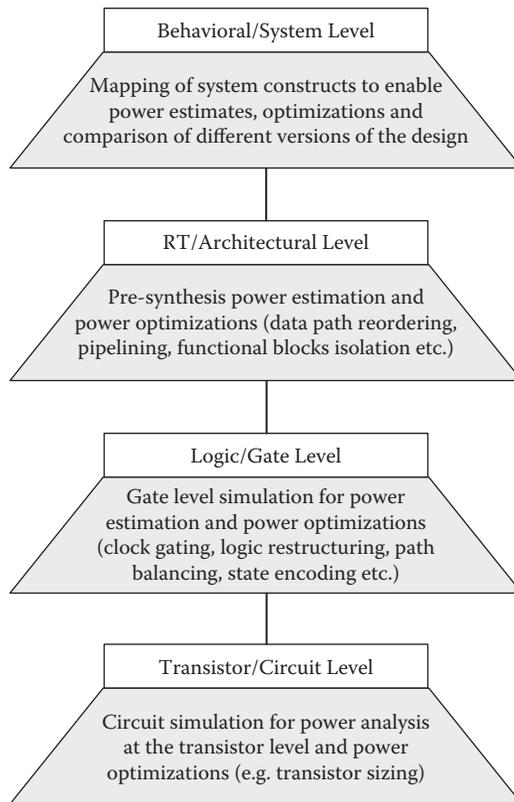
**Figure 10.7** Power-oriented design flow with power analysis and optimization steps.
