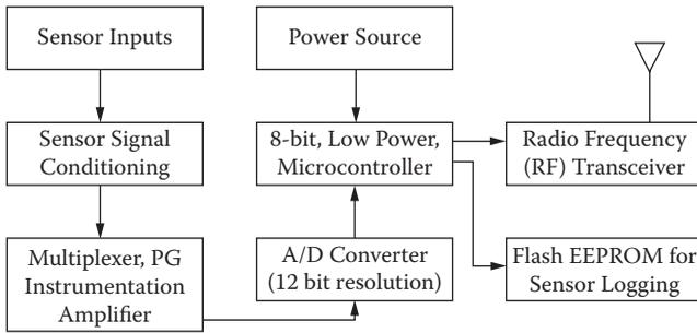
**Figure 10.1** A block diagram of a typical wireless microsensor node.
