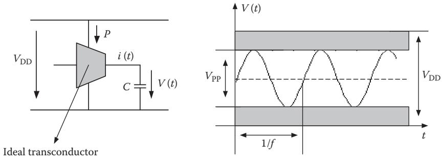
**Figure 10.3** An ideal, single-pole analog processing filter.
