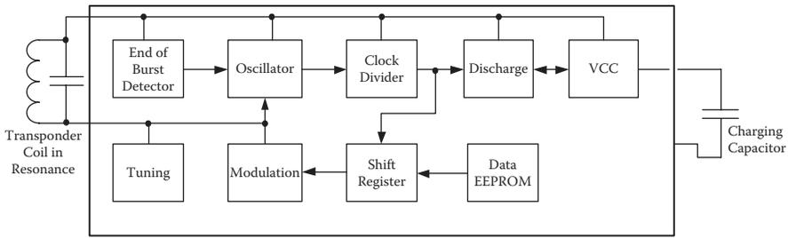
**Figure 10.2** Typical block diagram of an RFID tag.
