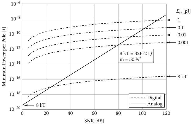
Figure 10.4 Minimum power consumption of analog and digital circuits.
