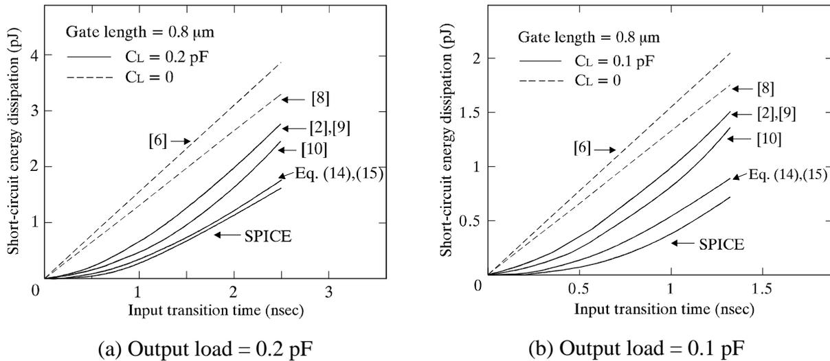
**Fig.3:** Short-circuit energy dissipation of a CMOS inverter per one clock cycle
