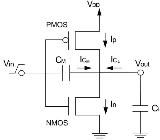
**Fig.1:** The CMOS inverter
