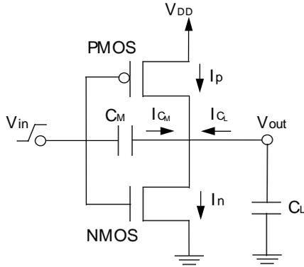
Fig.1: The CMOS Inverter
