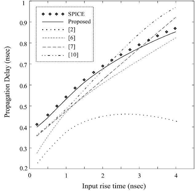
**Fig.5:** Inverter propagation delay
