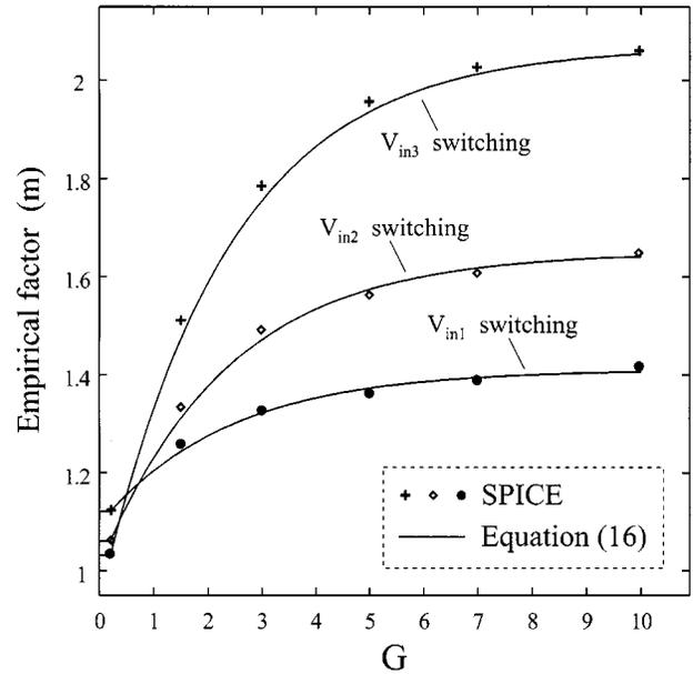
Fig. 8. Empirical factor  $m$  as a function of  $G = (I_{DON}\tau)/(V_{DD}C_L)$  for a three-input NAND gate.
