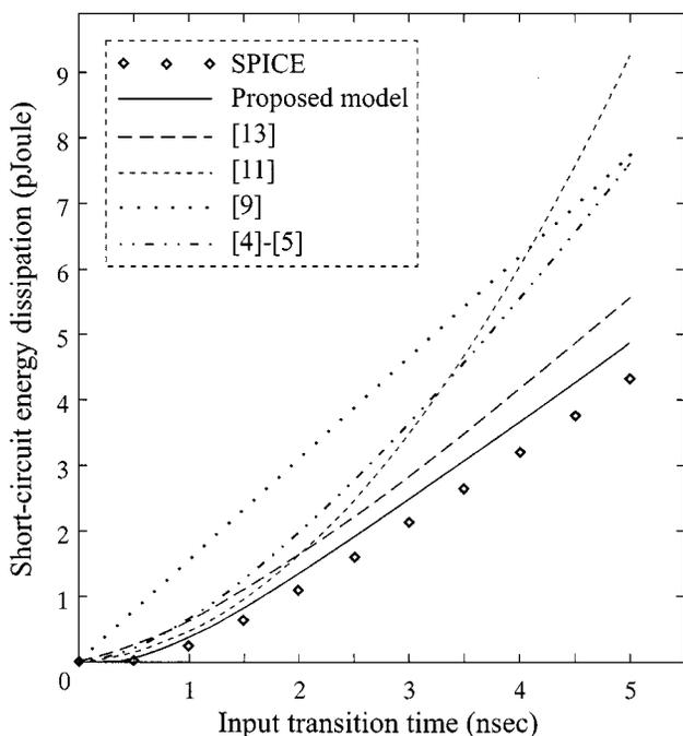
Fig. 10. Inverter short-circuit energy dissipation during one switching cycle, as a function of input transition time.
