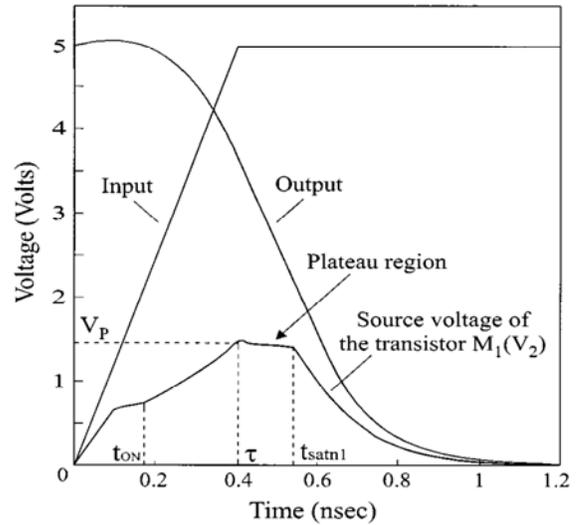
Fig. 6. Voltage waveforms of a three-input NAND gate for fast inputs.
