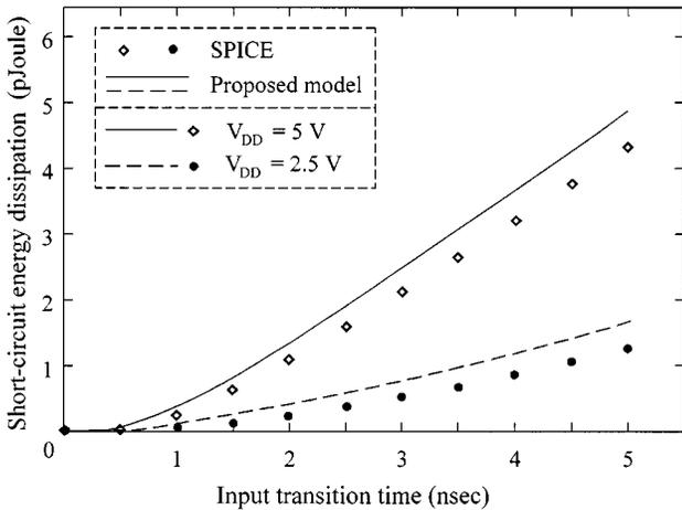
Fig. 12. Inverter short-circuit energy dissipation during one switching cycle, for two values of supply voltage ( $V_{DD} = 2.5$  V,  $V_{DD} = 5$  V).
