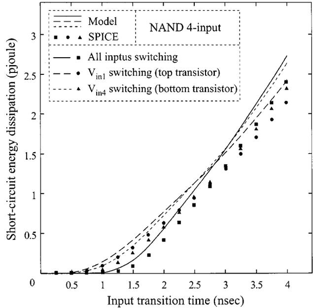
Fig. 14. Short-circuit energy dissipation of a four-input NAND gate during one switching cycle, as a function of input transition time.
