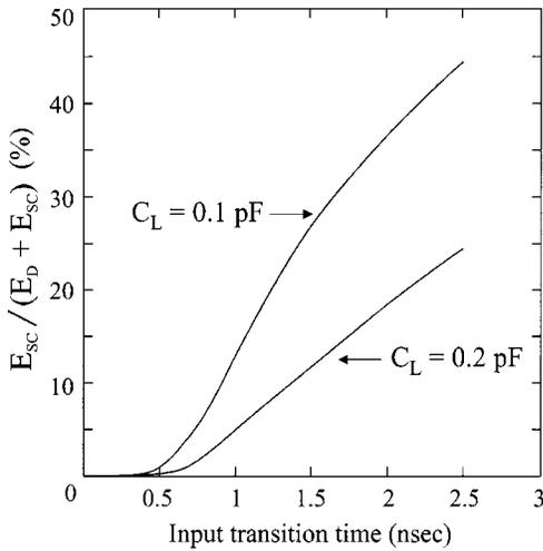
Fig. 11. Inverter short-circuit energy dissipation (a) and contribution of the short-circuit energy to the total energy dissipation (b) during one switching cycle, for two values of output load ( $C_L = 0.2$  pF,  $C_L = 0.1$  pF).
