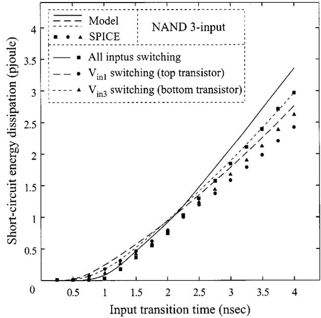
Fig. 13. Short-circuit energy dissipation of a three-input NAND gate during one switching cycle, as a function of input transition time.
