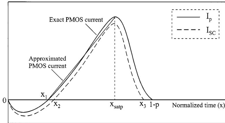
Fig. 4. PMOS and short-circuit current waveforms of the inverter.
