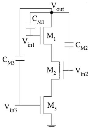
Fig. 9. Contribution of series-connected transistors (when they operate as short-circuiting block) to the gate equivalent input-to-output coupling capacitance.
