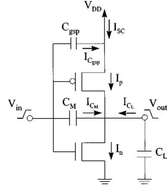
Fig. 1. The CMOS inverter.
