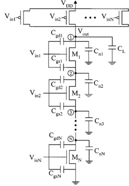
Fig. 5. Multiple-input static CMOS gate.
