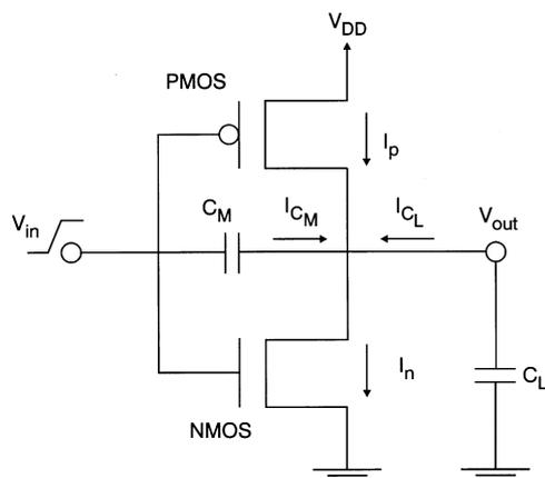
Fig.1 CMOS inverter
