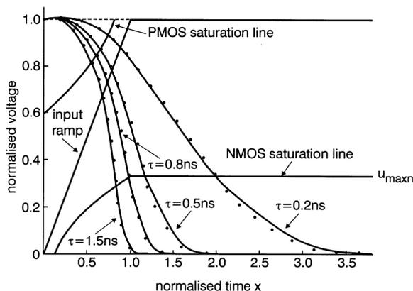
**Fig. 5** Inverter output waveforms for several values of input rise time
