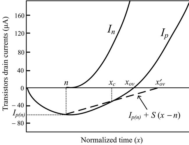
Fig. 7. Transistors drain currents during the early part of inverter switching process. The linear approximation of the PMOS current in order to obtain an output voltage waveform expression for  $n < x \leq x_{ov}$  is indicated.
