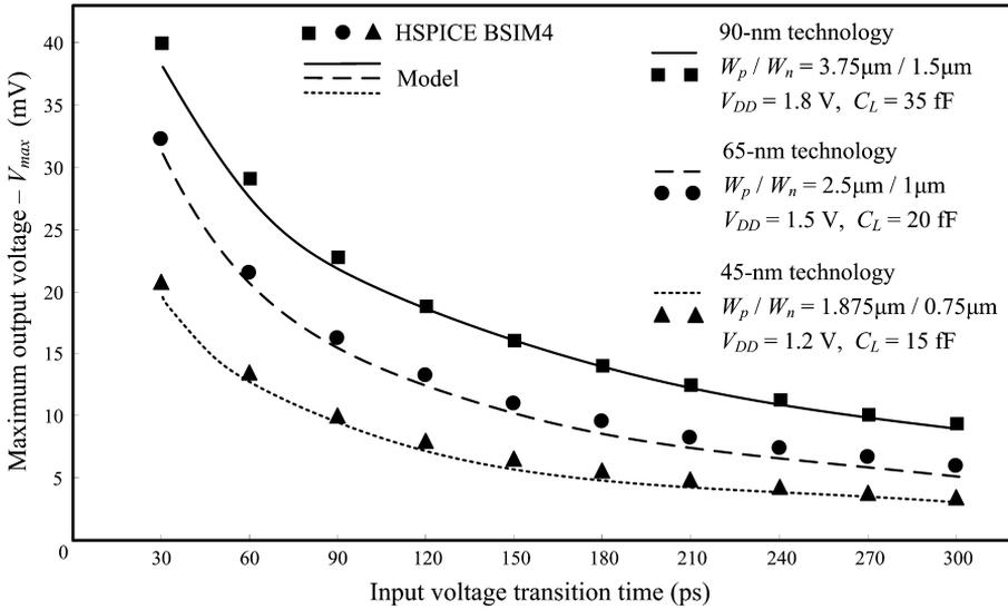
Fig. 11. Maximum output voltage obtained from the presented model as a function of input voltage transition time and comparison with BSIM4 HSPICE simulations for three different sub-100 nm technologies, transistor widths, output loads and supply voltages.
