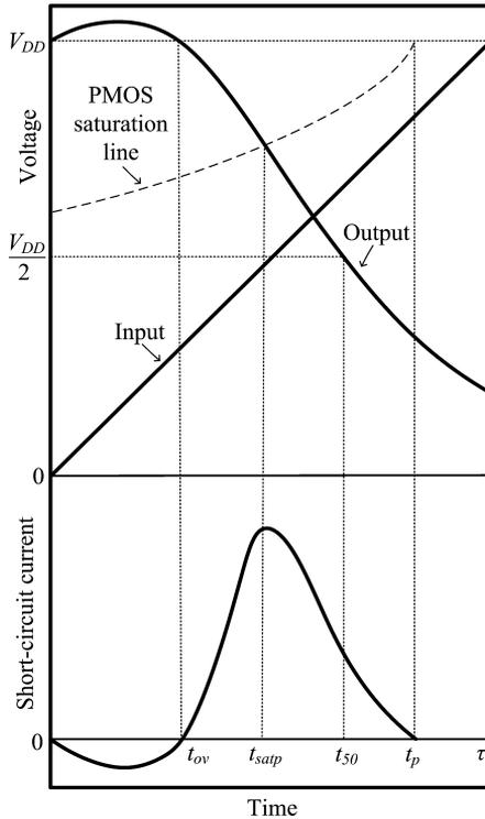
Fig. 2. Output voltage and short-circuit current of the CMOS inverter for a rising input voltage.
