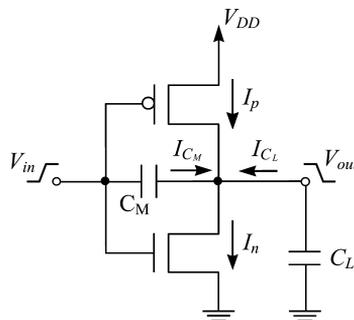
Fig. 1. The CMOS inverter.
