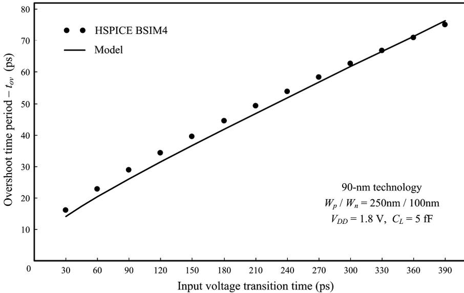
Fig. 10. Overshoot time period obtained from the presented model as a function of input voltage transition time and comparison with BSIM4 HSPICE simulations for narrow transistor widths.
