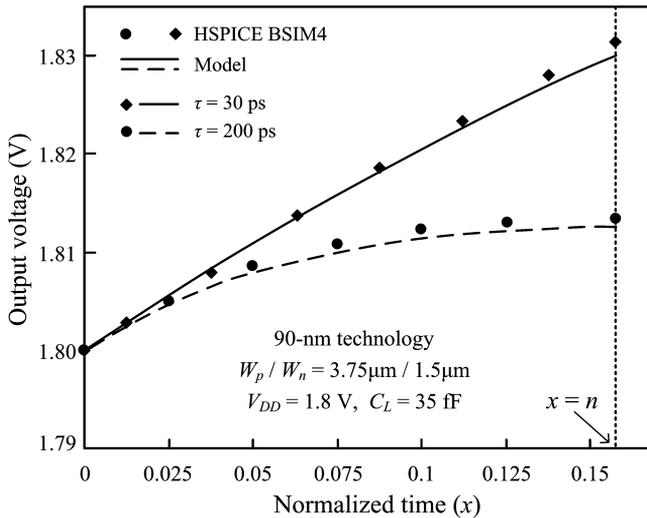
Fig. 6. Comparison of output voltage waveforms derived by Eq. (12) (for  $0 \leq x \leq n$ ) with those produced by HSPICE BSIM4 simulations, for two different input transition times.
