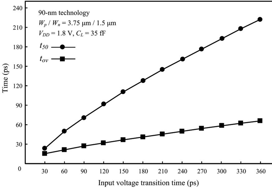
Fig. 3. Overshoot time period ( $t_{ov}$ ) and time period for the output voltage to reach 50% of the supply voltage ( $t_{50}$ ), as a function of input voltage transition time in a CMOS inverter.
