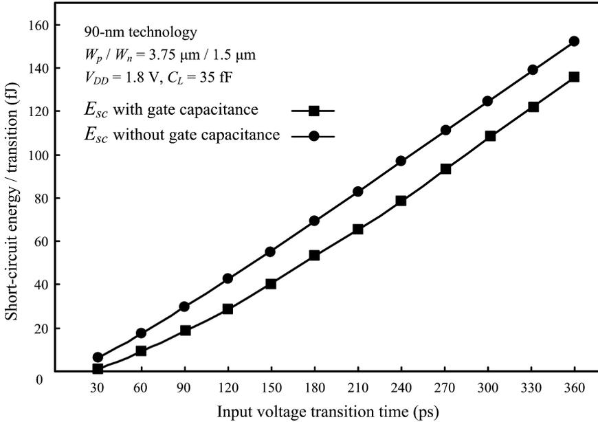
Fig. 4. Short-circuit energy dissipation per transition ( $E_{sc}$ ) with and without the influence of transistors' gate capacitance, as a function of input voltage transition time in a CMOS inverter.
