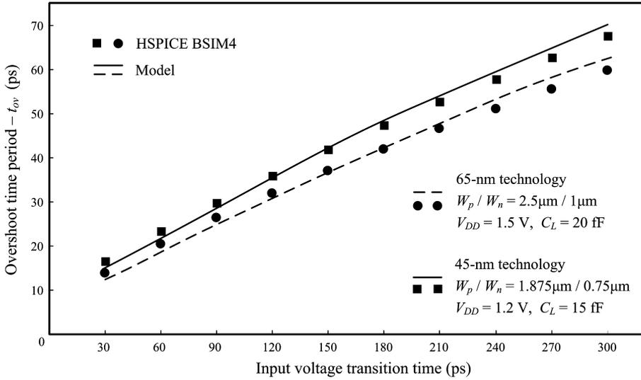
Fig. 9. Overshoot time period obtained from the presented model as a function of input voltage transition time and comparison with BSIM4 HSPICE simulations for two different sub-100 nm technologies, transistor widths, output loads and supply voltages.
