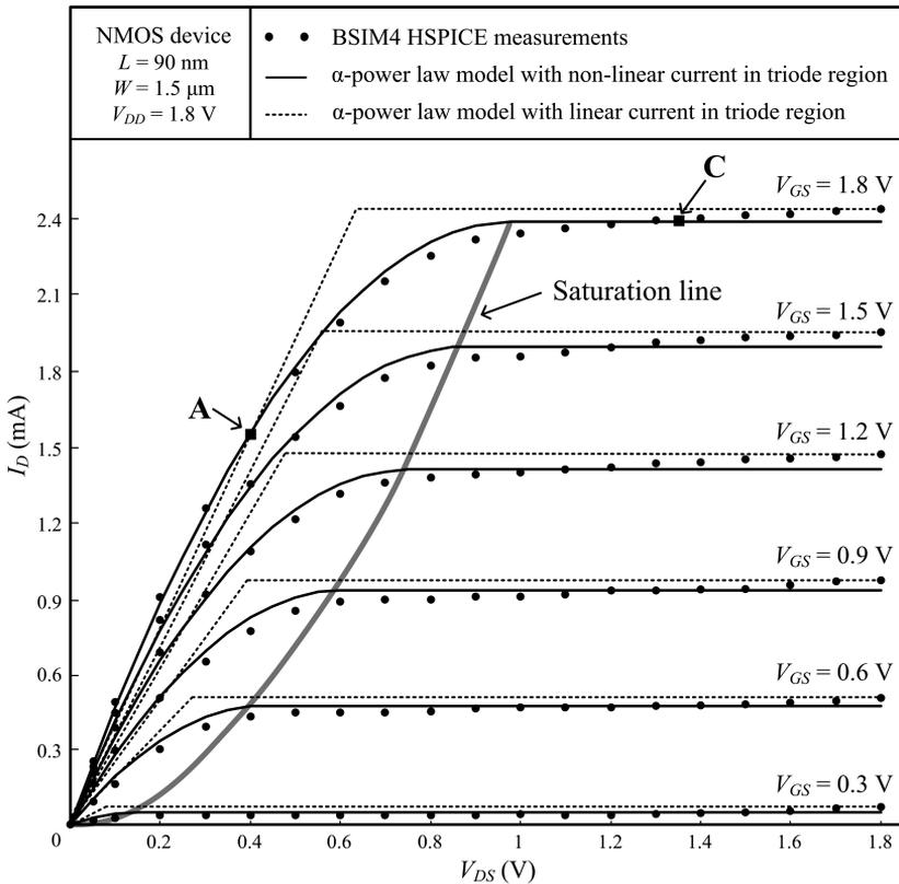
Fig. 5. 90-nm NMOS device  $I$ – $V$  plots.
